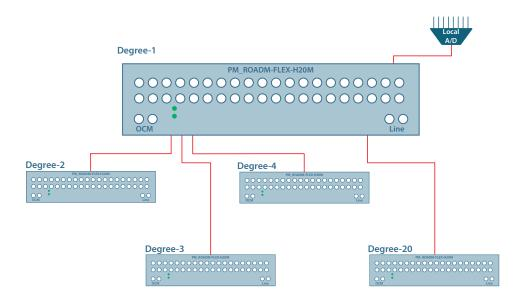
Figure 1: Twenty degree network architecture using PM ROADM-FLEX-H20M
